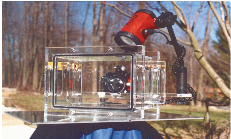
Figure 11.3.48 Camera with a Clear Box
